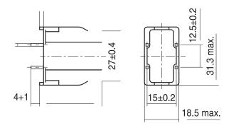
Part tolerances to ISO 2768-cL / ISO 8015. Size ISO 14405 (E) All dimensions in mm
