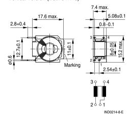
Tolerances to ISO 2768-M unless otherwise noted. Dimensions in mm.
